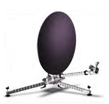
The unique shape and the accurate reflector surface provide good sidelobe and cross polarization performance. Repeatability is maintained with precision registration of the 6 reflector segments and the feed support structure. All the models are provided with a 2-Port Feed as a standard. In Dual and Tri-Band configuration the Feeds are interchangeable on field, fast and No-Tools.
